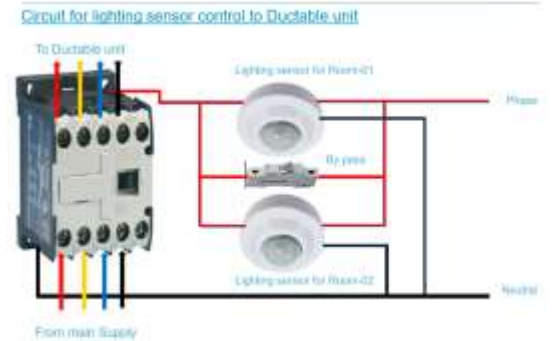
Auto operation of AC unit via motion sensors
